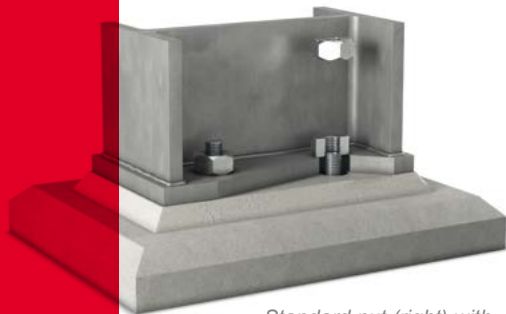
Standard nut (right) with insufficient anchor rod
