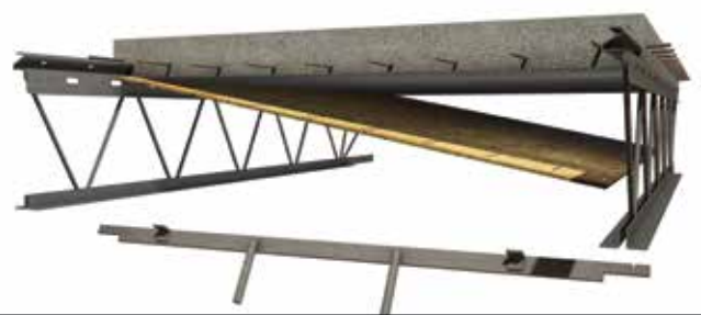
6- Removal of plywood forms
