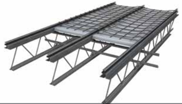
4- Sheets of mesh
