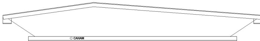
The Canam-Joist-2Slope family allows for the creation of one (1) Top Chord ridge. The Ridge Depth distance is calculated from the Bottom Chord (parallel to the BC). The Ridge Offset distance is calculated from the Joist Start position. When the Ridge Offset parameter is set to 0", the Ridge Offset distance is located in the middle of the joist length.
