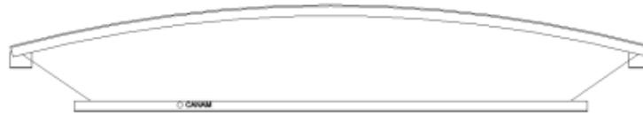
The Canam-Joist-Bowstring family allows for the creation of an arched Top Chord. The TC Radius is always calculated perpendicular to the plane that passes through the Joist "Working Points" (Placement Points). The user can specify the Top Chord Radius distance by inputting a value in the TC Radius parameter.
