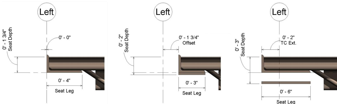
The Start Offset and the End Offset parameters are used to position the joist ends from the axis. The Joist Seat position is calculated according to the Offset value. The TC Extension parameter is also used to position the joist ends from the axis.
